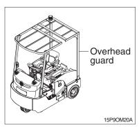
(1) The head guard is of rugged construction that serves to ensure the safety of the operator.
